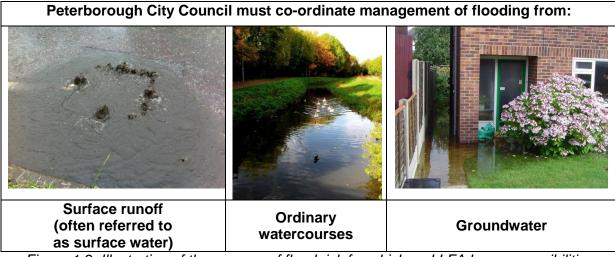
Figure 1-2: Illustration of the sources of flood risk for which an LLFA has responsibilities
